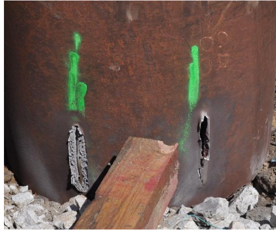
Figure 5-4. Prediction markers and impacts. The rough order of magnitude predictions actually predicted where the liner fragments would impact the pipe.
