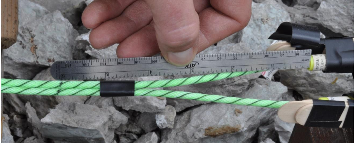
Figure A. 7: Mark the sections of det-cord so that length of det-cord from the booster to the mark is equal on both sides
