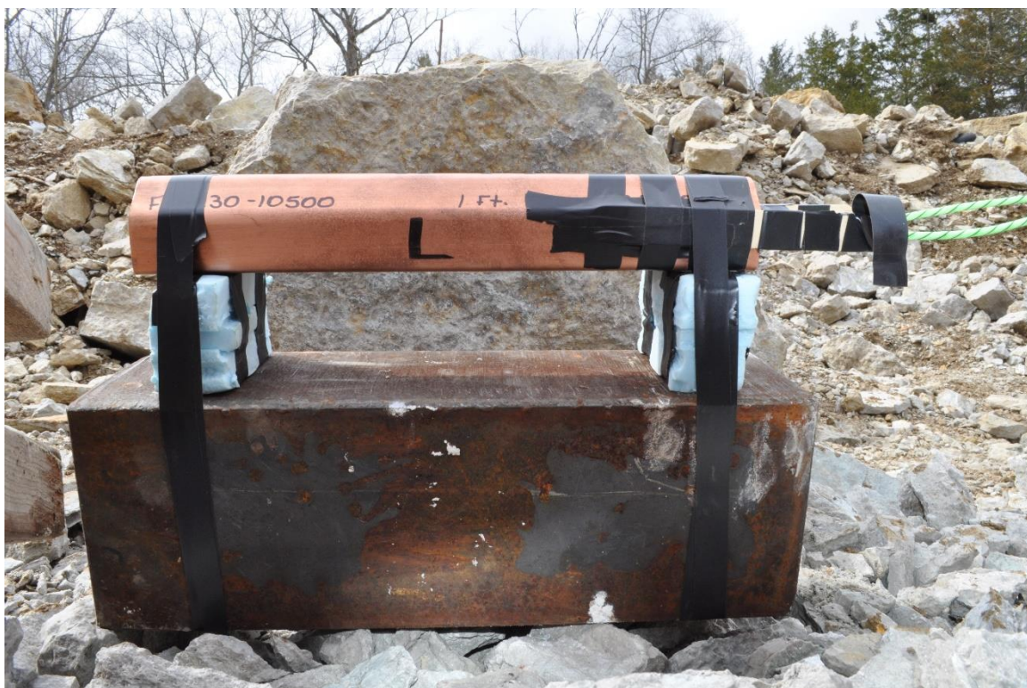
Figure A. 6: Secure the dual initiation system and LSC to the target at the desired stand-off distance
