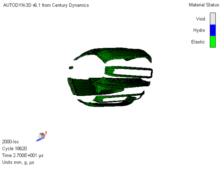
Figure 2-6. LSC 27 \mu sec after detonation (Lim, 2006). By this time the explosive has accelerated the entire length of the LSC liner. Notice how all the faces have been projected outwards (when compared to figure 2-5) and the blade has almost completely formed from the collapse of the LSC legs.
