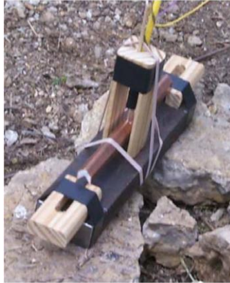
Figure 3-6. Midpoint initiation test setup (Lim, 2003). For this initiation method started the detonation in the center of the LSC via a hole that was drilled through the liner. This method was developed based on the idea that cut dynamics of a LSC was similar to a CSC.
